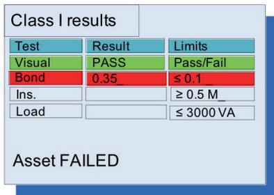
The screenshot shows a window titled 'Class I results' containing a table with three columns: 'Test', 'Result', and 'Limits'. The 'Bond' test row is highlighted in red, indicating a failure. Below the table, the text 'Asset FAILED' is displayed.
